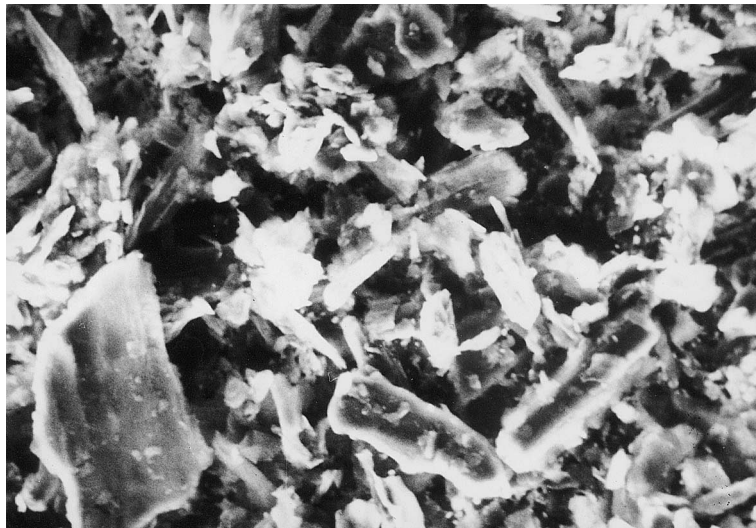
Fig. 2. SEM micrograph of graphite EG particles (magnification 500×).
